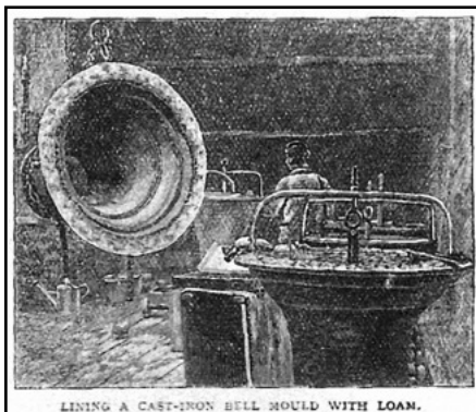
LINING A CAST-IRON BELL MOULD WITH LOAM.
